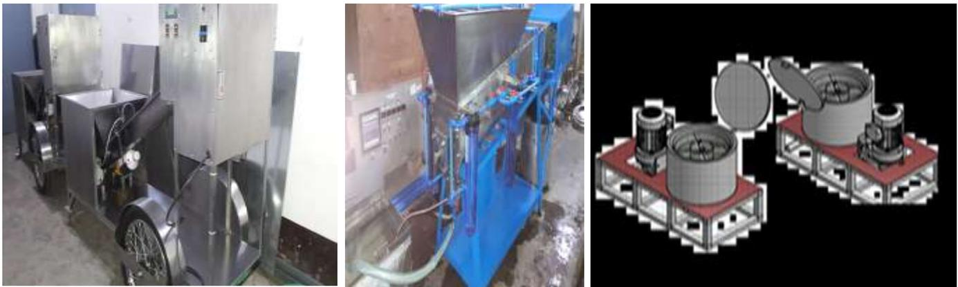
**ITDI's Salt Iodizing Machine (SIM).** *Left to right. Frame 1: Salt Iodizing Machine – Continuous Type. Frame 2: Salt Washer. Frame 3: Spin Dryer.*
