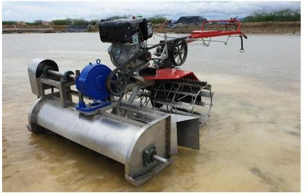
procedures in a deep crystallizer saltern. It makes salt processing possible during dry and wet seasons and eliminates the laborious crushing, piling, and hauling of salt by hand using rakes, barrows, and pushcarts. The automated process reduces the harvesting process from months to weeks, thus reducing
