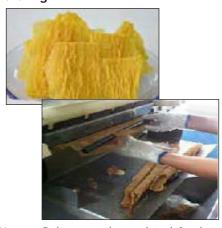
Mango flakes are drum-dried fresh mangoes (Carabao variety) at its optimum maturity (rare ripe with peel color of 80 percent yellow and 20 percent green), with firm texture. Drum drying is a continuous, indirect drying method that allows short retention time while evaporating all the liquid in the product within a single rotation of the drums.
