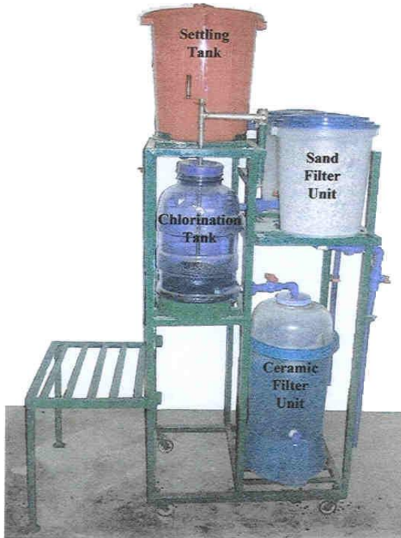
Fig. 1. The locally fabricated small-scale water purification system
