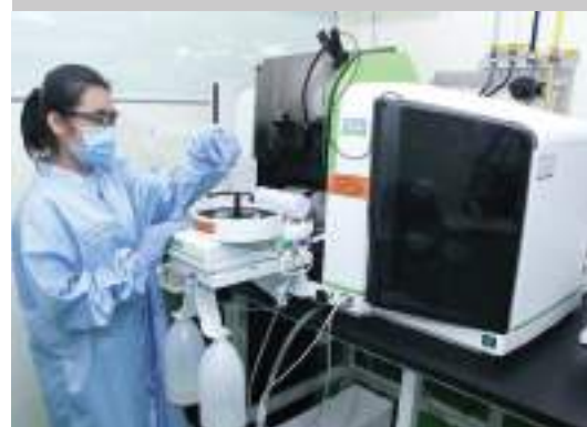
Analysis of trace metals in PT samples using Flame Atomic Absorption Spectrophotometer
