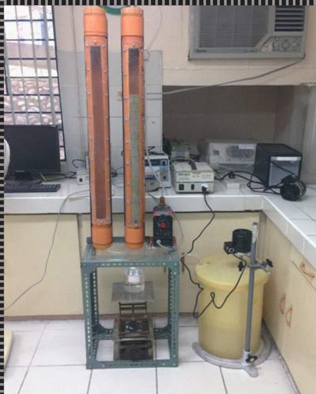
Column testing of surface-modified zeolite using diesel-contaminated wastewater
