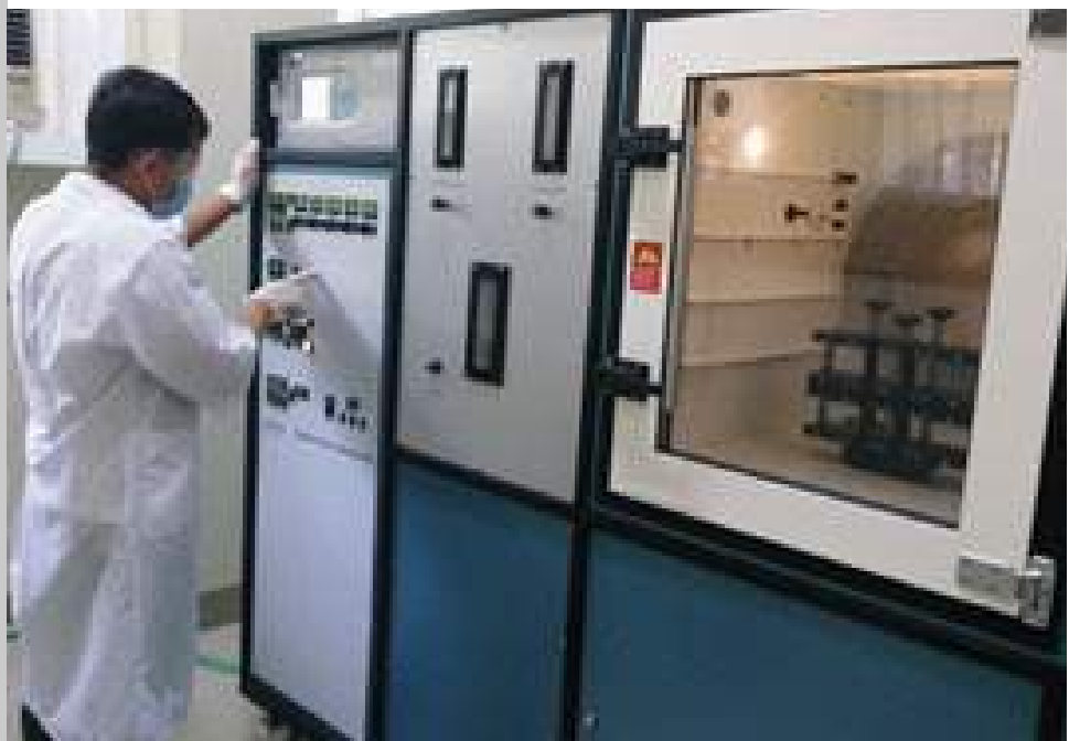
Testing of rubber product using ozone chamber
