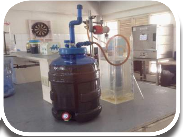
Treatment for 18 L contaminated waste water with Cu (Anaerobic Conditions)
