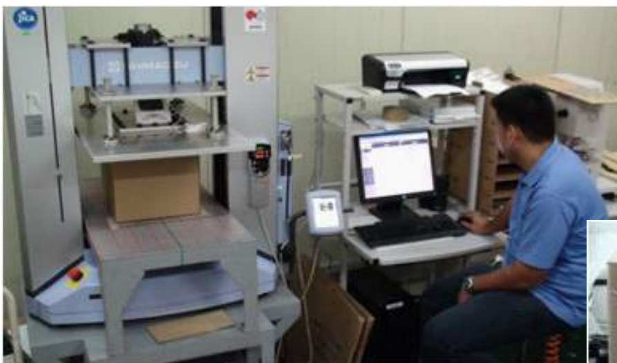
Compression testing using PTD's Shimadzu AG-X Testing Machine
