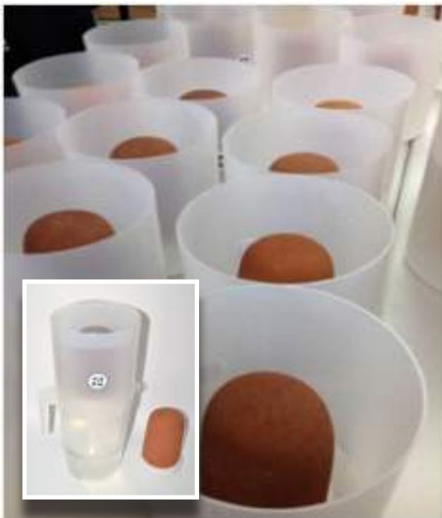
Candle-type ceramic water filter system
