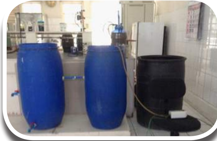
Treatment for 80 L contaminated waste water with Cu (Aerobic Conditions)
