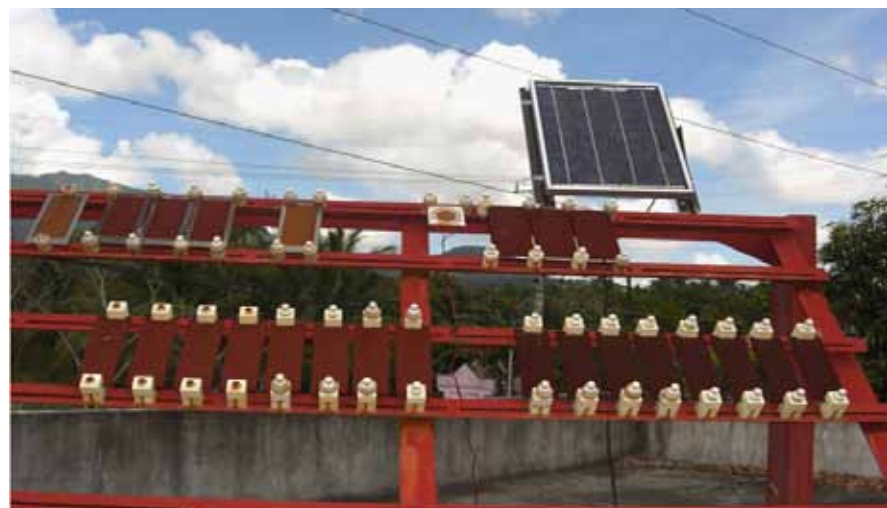
Exposed Test Panels with ACM Sensor in Bay, Laguna
