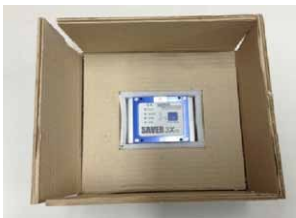
Data recorder used for measuring vibration shock during transport
